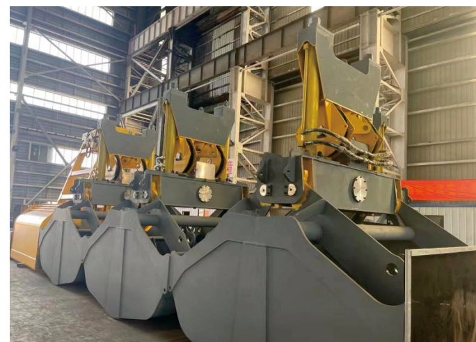
Visual on grab body after sand blast
