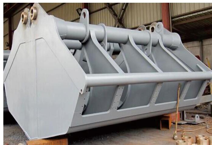
Visual on grab body after sand blast
